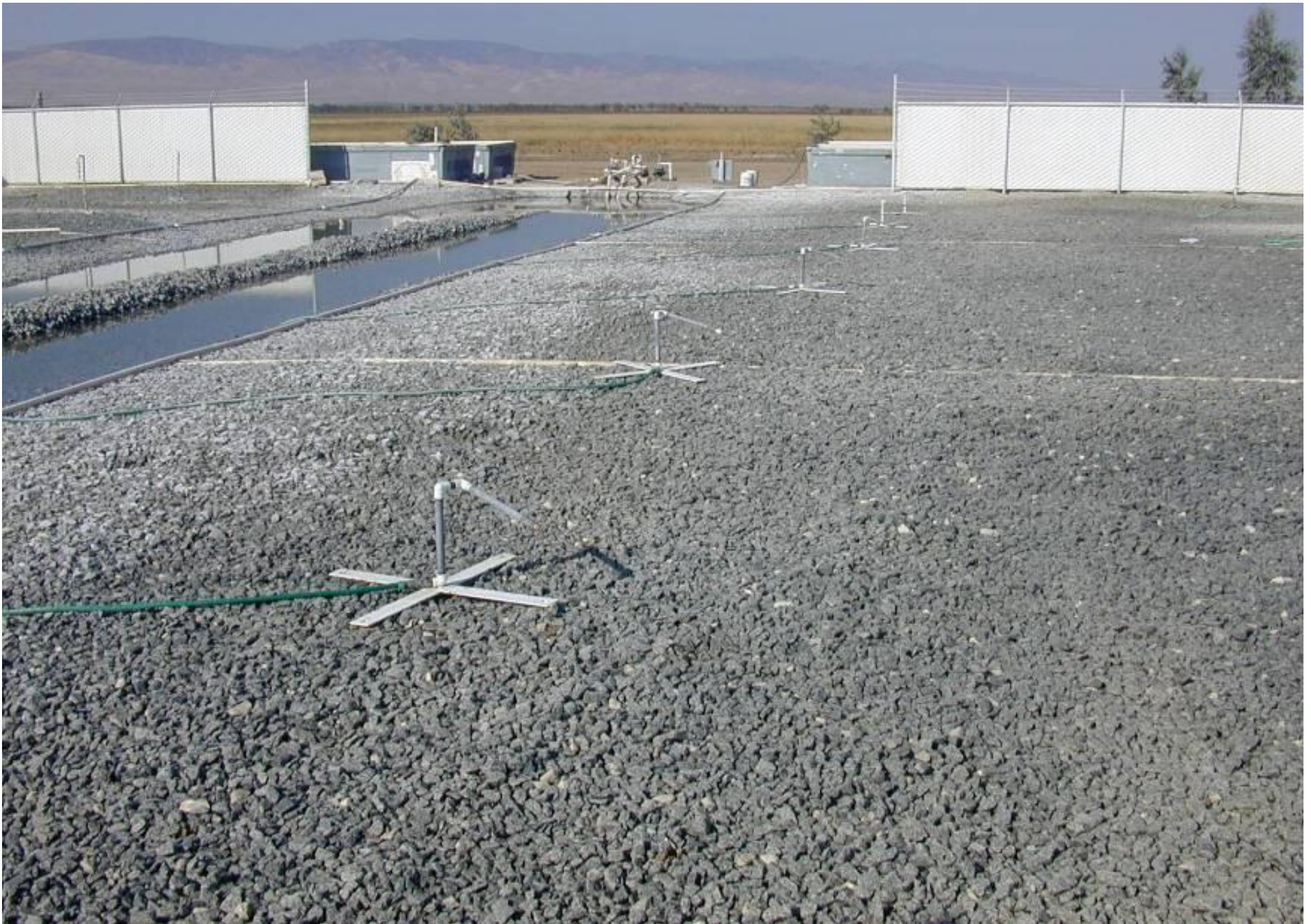
Nozzle positions with different angles and with varying riser heights were tested in 2003 (riser=1.0 ft)
