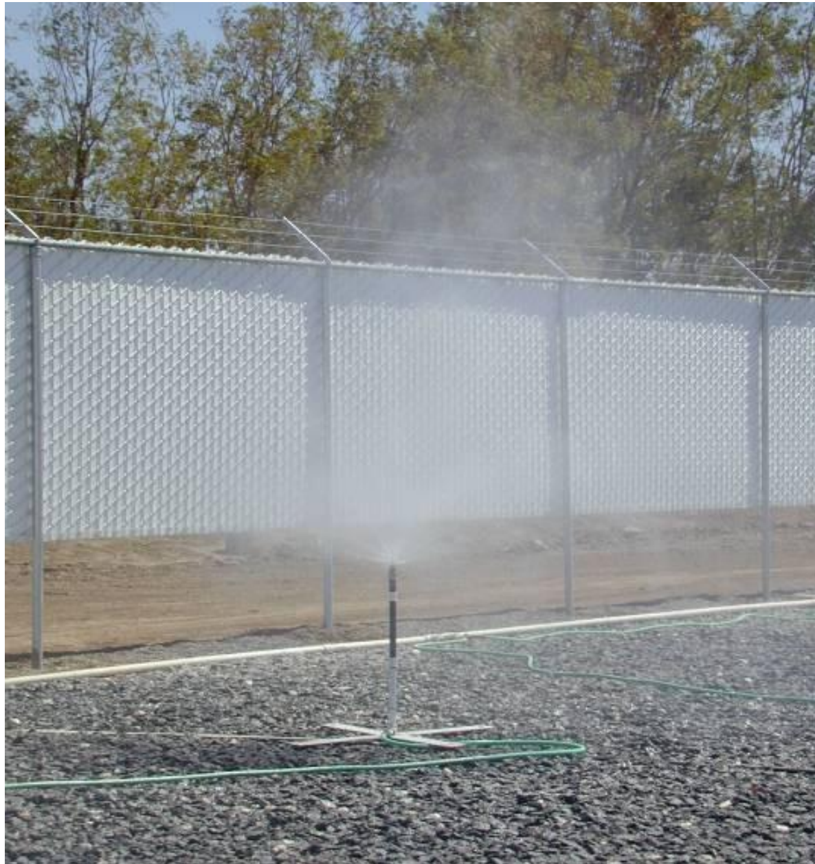
Vertically oriented nozzle position with different riser heights (riser=1.5 ft) note windbreak fence
